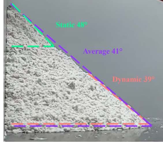
Figure 3. Static, dynamic and average angle of repose of a representative LLD-1 sample.
