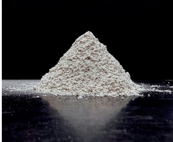
Figure 1. Lunar low-density (LLD-1) regolith simulant.
